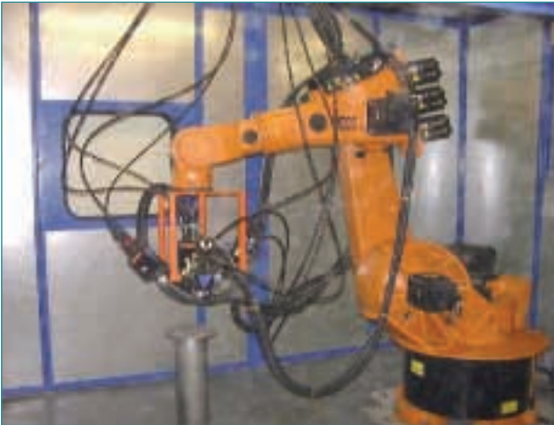
Above: The sprayforming apparatus for the manufacture of tools and dies, located at the University's Begbroke Business and Science Park.
