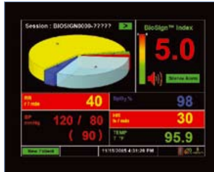
BioSign display at the time of an alert: the five parameters are the respiratory rate (RR), the blood pressure (BP), the oxygen saturation level ( \text{SpO}_2 ), the heart rate (HR) and the skin temperature (temp). The pie chart indicates that the most abnormal parameter is the respiratory rate (in yellow), followed by the heart rate (in grey).
