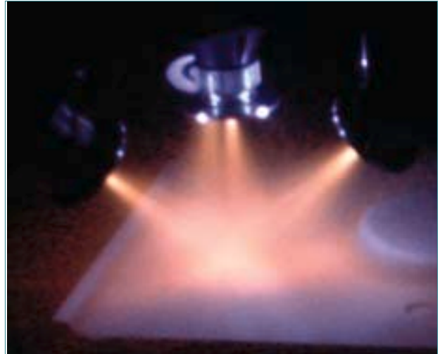
Above: Thermal sprayforming of development tool for Airflow Streamlines plc by Novarc
